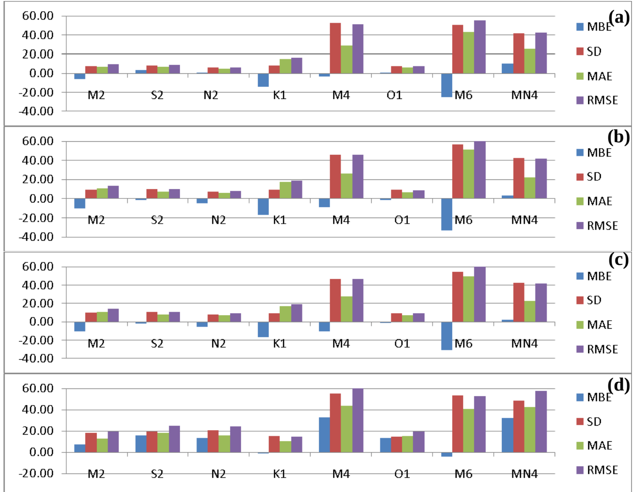
Figure 5.4: Four 2D phase error measures, mean bias error (MBE), standard deviation (SD), mean algebraic error (MAE), and root mean square error (RMSE), for each of 8 water level harmonic tidal constituents for the (a) 2DCR, (b) 2DNR, (c) 2DRR, and (d) 2DBF experiments.
