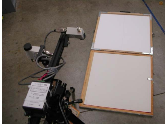
Figure 34 Image of the Avalanche Photo-Diode Setup
