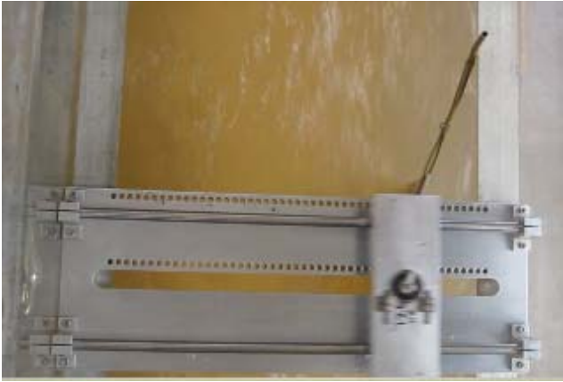
Figure 7. Oscillator moment arm contacting the wall.
