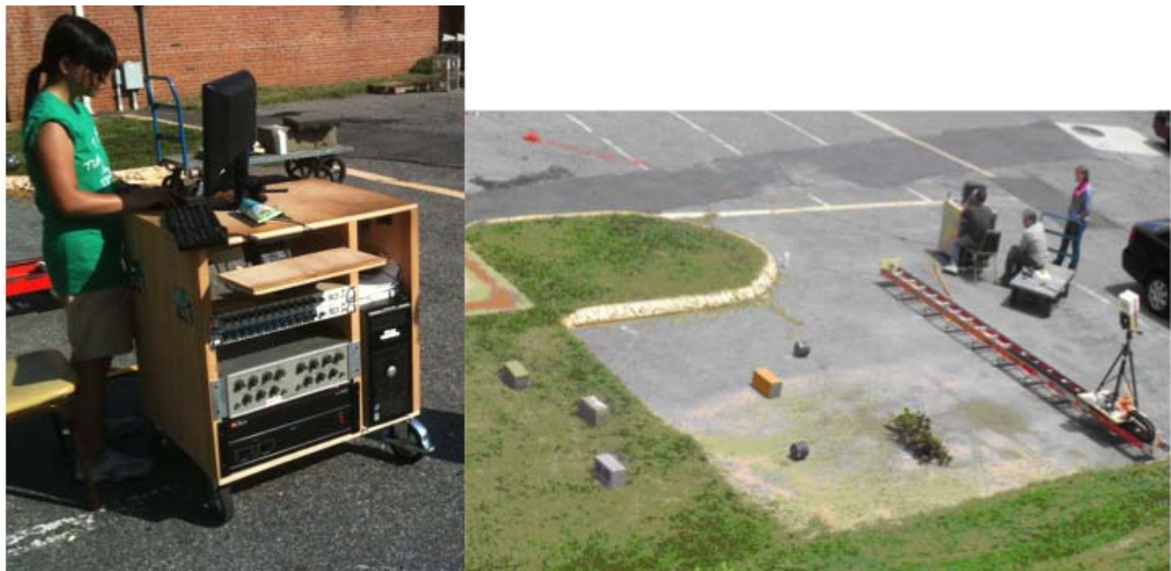
Figure 2 The photograph on the left shows an operator initiating a data collection from the mobile rack. The photograph on the right shows a typical experimental configuration where a number of targets are arranged within the measurement field of the SAA system.
