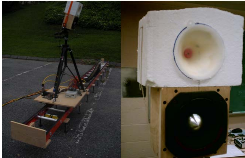
Figure 1 is a photograph of the SAA measurement system mounted on a 6.3 m rail. The transceiver is mounted on a tripod that is supported by a motorized platform that traverses the rail. The inset is a close up view of the acoustic transceiver.
