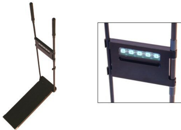
Figure 8. Illuminator node showing IR LED package housing an array of five LED clusters on both sides.
