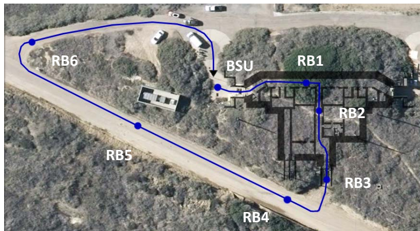
Figure 11. Travel path of the PackBot carrying the APDS system showing deployed locations of the NG Relay Bricks through the WWII bunker and around the hill, with threshold level set to 45. Black triangle at top center shows the final location of the PackBot.
