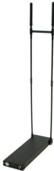
Figure 6. Next Generation Relay Brick with raised antennas that are 24" above ground.
