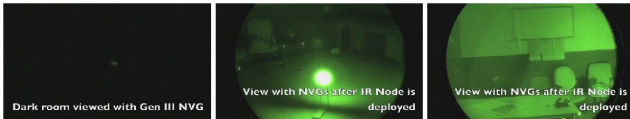
Figure 13. Before (left image) and after (center and right) images of the illuminated room. Center image shows direct view of Illuminator Node. Right image shows a better representation when not directly viewing the IR LED source.
