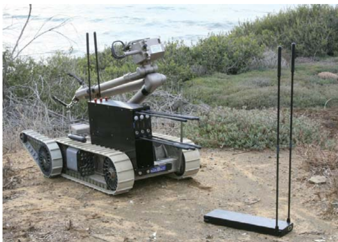
Figure 9. EOD PackBot carrying the APDS Deployer containing three stowed NG Relay Bricks and one deployed with raised antennas.
