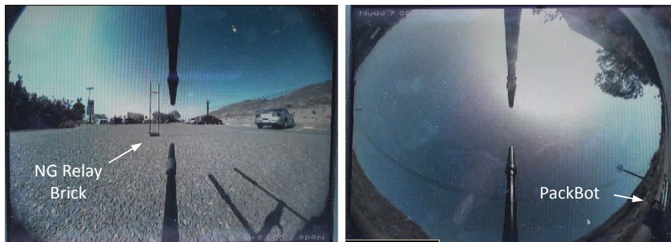
Figure 12. Screenshots of the video received from the Camera Node when stowed (left image) and when deployed (right image).
