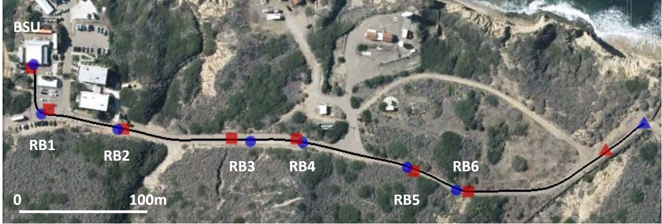
Figure 10. Travel path of PackBot showing deployed locations of NG Relay Bricks (RB1 to RB6) and final position of PackBot (triangle) with a threshold setting of 45. Blue disks and red boxes indicate deployed locations under “normal” and “fast” speed modes, respectively.
