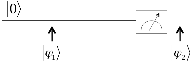
Figure 3.1: Single qubit circuit with no Identity gate
