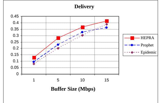
Figure 5. HEPRA increases delivery when size of buffer increases
