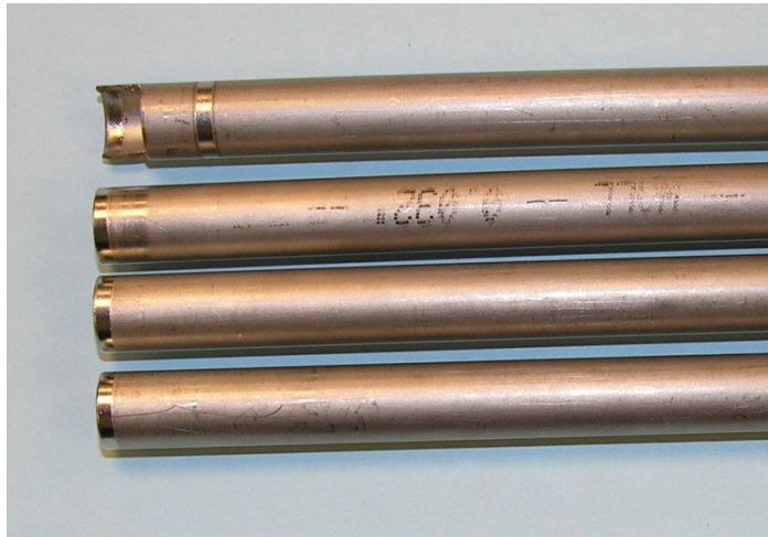
Figure 5 : Photograph of laser cleaned tube inner and outer edges.
