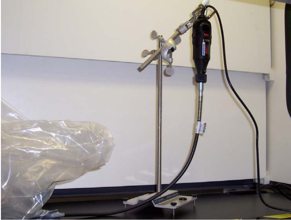
Figure 5 Dremel tool setup during cut experiments
