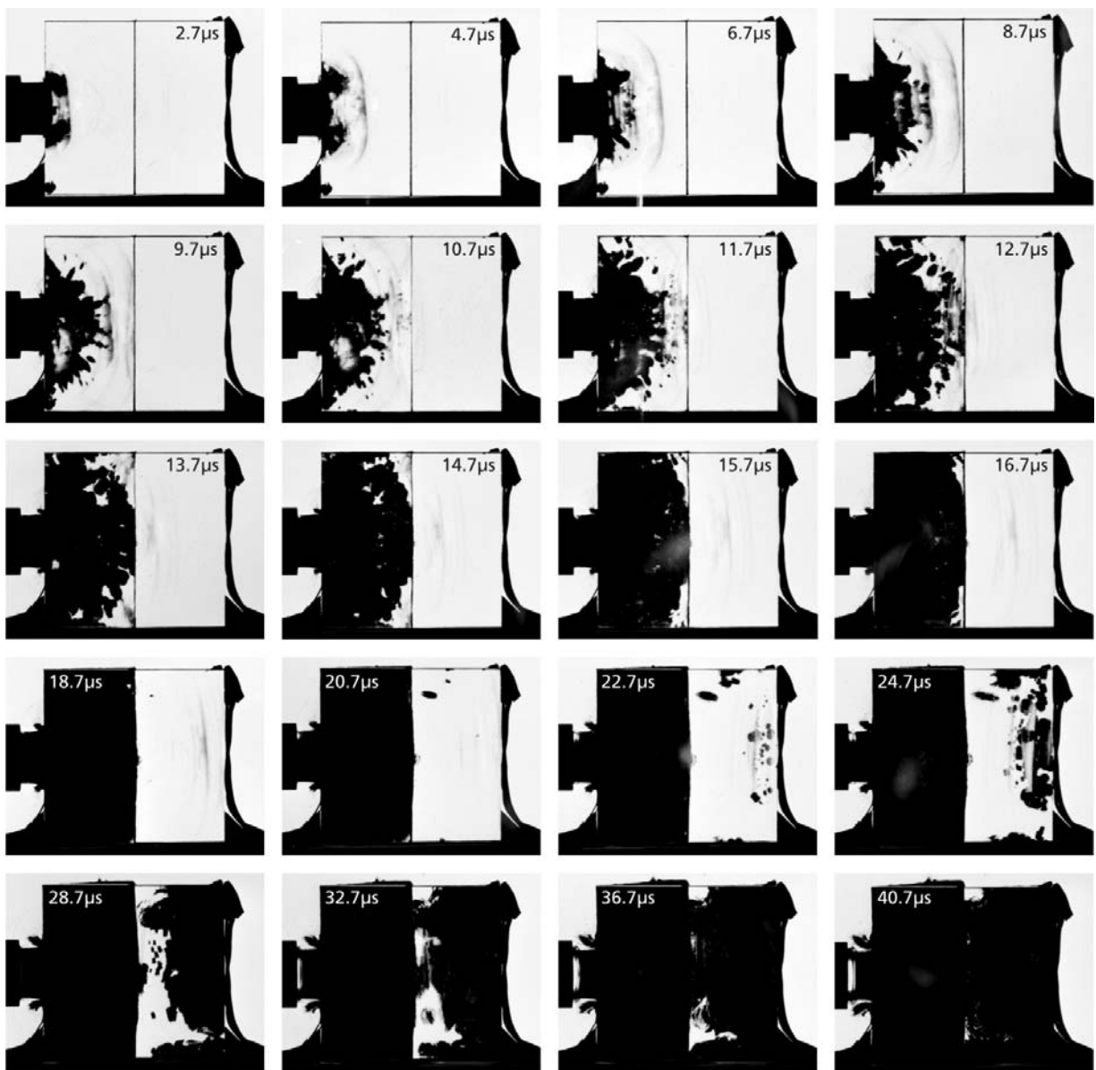
Figure A-14. Complete set of high-speed photographs from test with two-layer Starphire laminate at \approx 60^\circ\text{C} , cylindrical projectile, impact velocity 389 m/s, test no. 16588.
