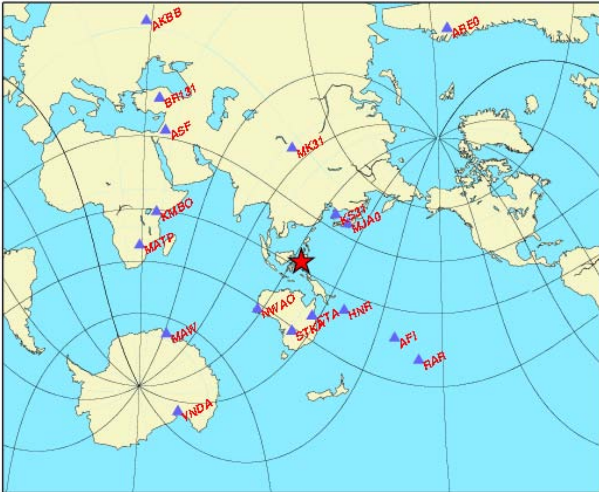
Figure 2. Map centered on the Celebes Sea event (red star) showing the location of the broadband stations (blue triangles) used in the MT inversion. Only associated SEL0 stations were used in this case. This result was obtained shortly after the event was written to the SEL0 database table.
