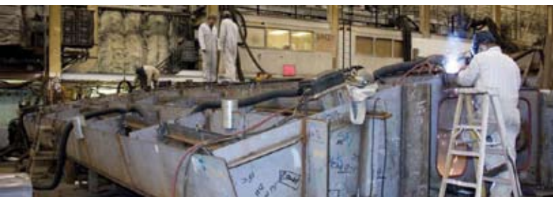
Workers at the General Dynamics-Bath Iron Works shipyard in Bath, Maine, weld together pieces of an inner-bottom unit for the future USS Zumwalt (DDG 1000). (Photo courtesy General Dynamics)
