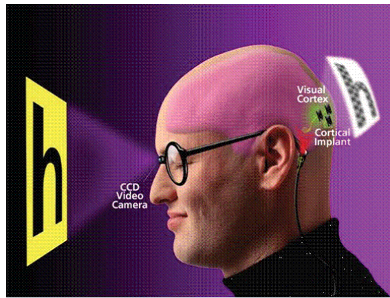
Illustration of a proposed artificial system featuring UEA implanted in the primary visual cortex.
