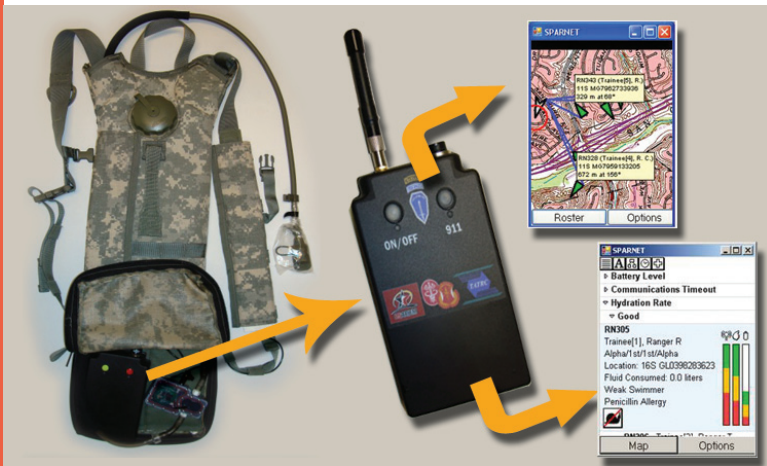
A hydration unit with integrated SPARNET radio/processing unit and USARIEM fluid intake monitor. SPARNET is a body-worn, software-defined-radio and physiologic-algorithm processing unit that integrates a BIONET inductive link to sensors, which report via a three-axis accelerometer and inclinometer, GPS receiver, and contains a battery-charge monitor.
