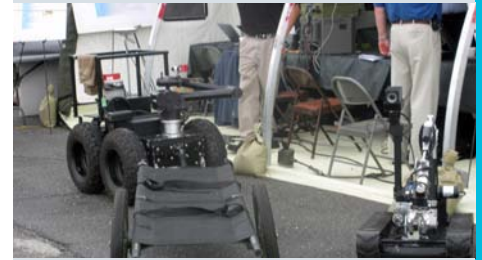
Robotic combat casualty assessment and extraction prototypes by Applied Perception Inc. (left) and American GNC (right).
