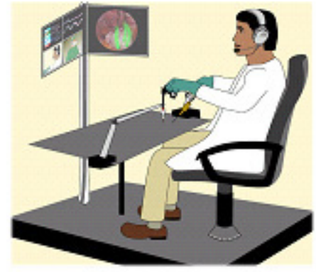
In the development of a haptic guidance system to facilitate minimally invasive surgical training and telerobotics, an expert surgeon's motions are recorded during a procedure (left). This data is used to develop a training simulation where novice surgeons practice by imitating the expert surgeon's gestures (right).
