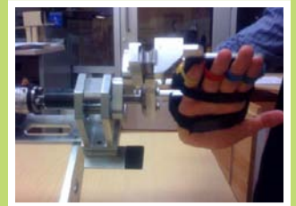
Right: A hand in the linkage, with emphasis on the 3 contact points and the Velcro straps that attach the fingers to the links of the exoskeleton. Below: The ARMinIII exoskeletal robot. Photo courtesy of the ETH and University of Zürich, Switzerland.
