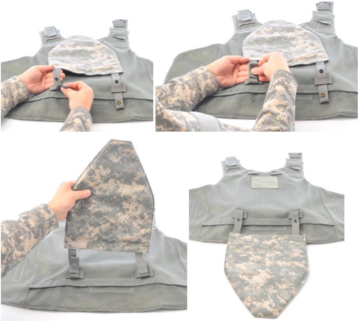
Figure D-3.24. Attaching Groin Protector.
