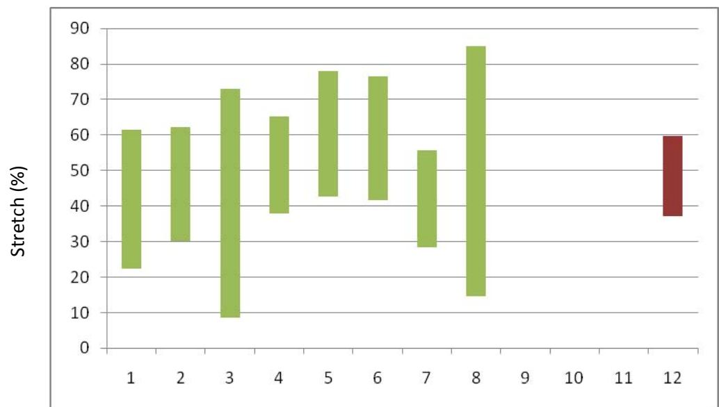
Chart 5. Waist Band Material Stretch Characteristics after 3 Wash Cycles
