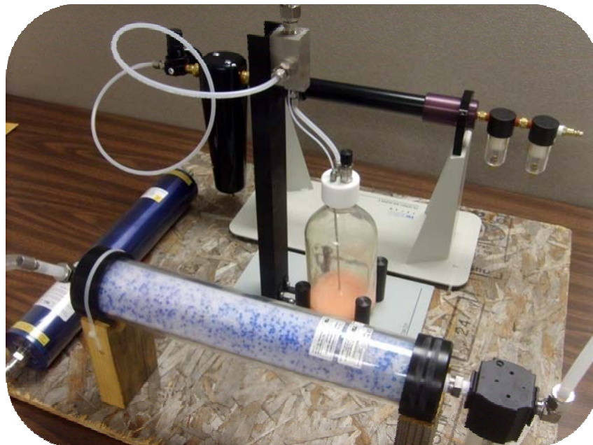
Figure 3. Assembled aerosol generation apparatus.
