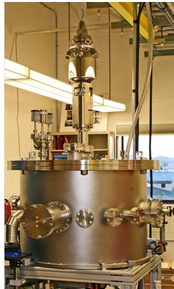
Figure 3. X-ray measurements using 100 keV electron source.
