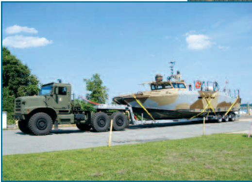
Above: A RCB on the first-article Hydraulic Boat Trailer, behind an MTVR Mk31 tractor at Aberdeen Test Center qualification tests.
