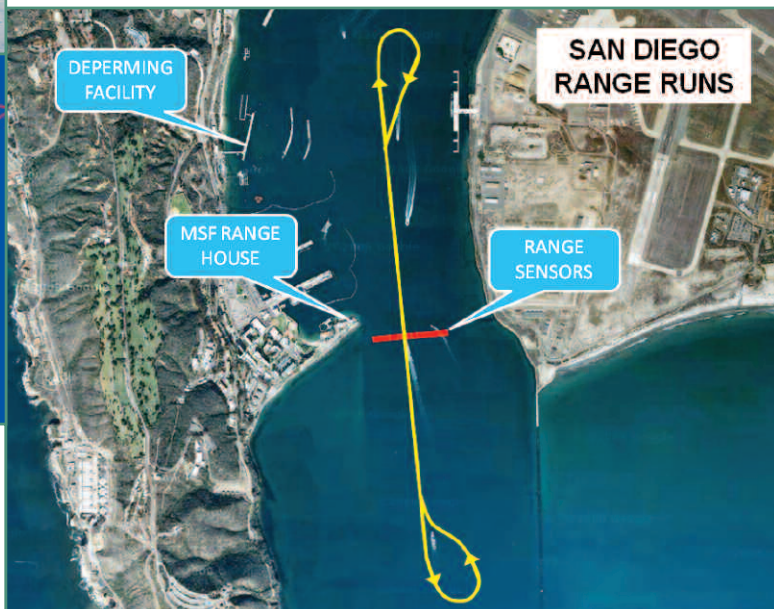
Above: Aerial view of the San Diego Magnetic Silencing Facility. The image shows the perpendicular approach and Williamson turn features of the range runs.
