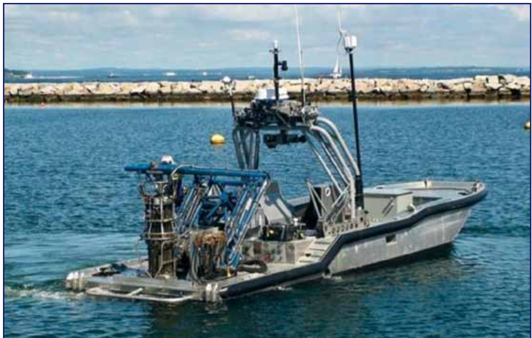
Above: An ASW USV configured with dipping sonar. Photo courtesy of NUWC Newport and PMS 403.
