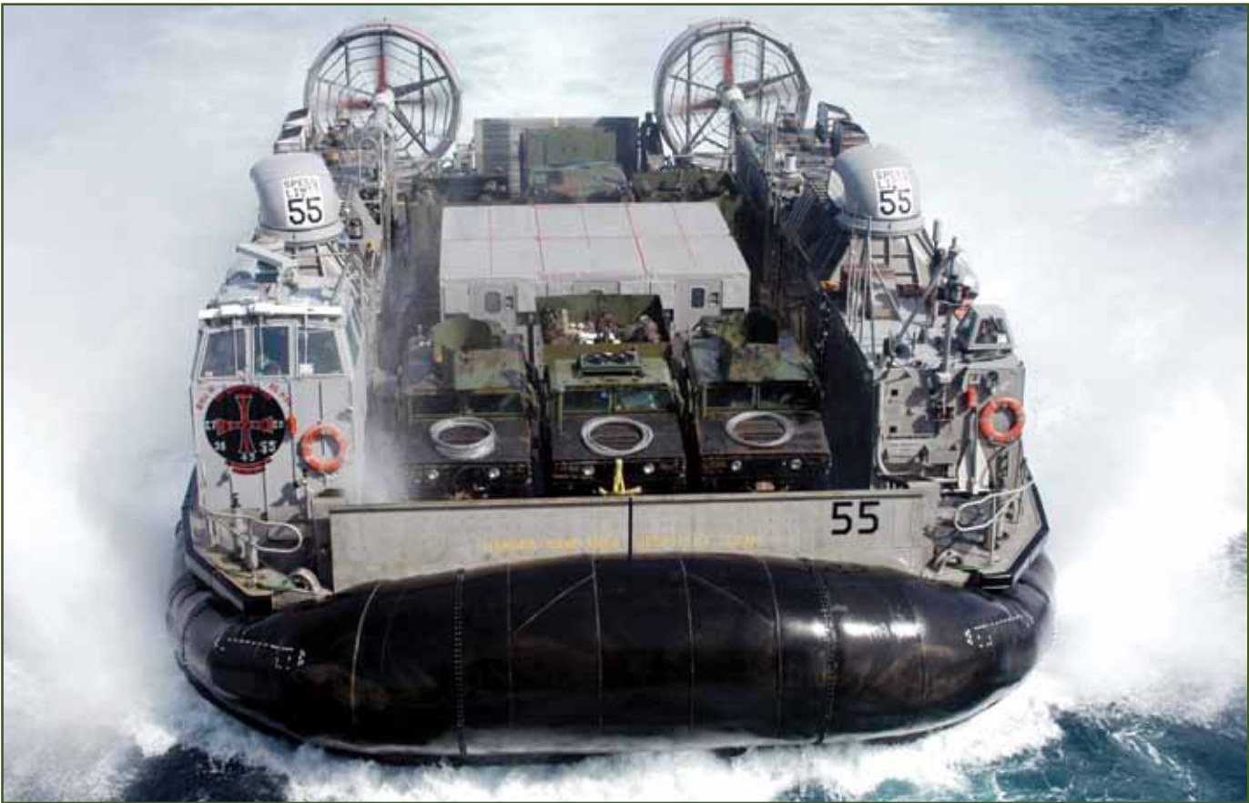
Above: LCACs like the one pictured above are currently in a life-extension program that will add 10 years to the vehicles' service life. There will be a significant need for the SSC once LCAC end-of-life component and material issues start to appear. U.S. Navy photo.
