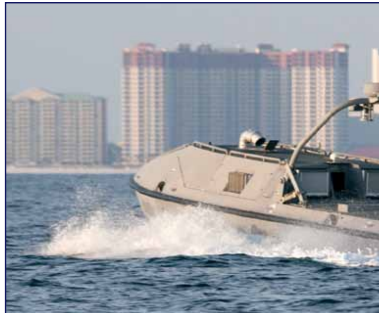
Above: MCM USV in transit. Photo courtesy of NSWC Panama City and PMS 403.
