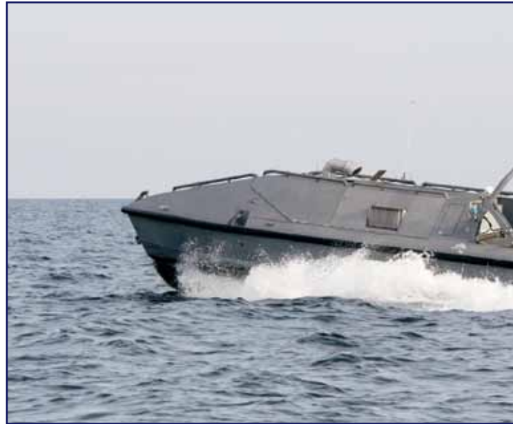
Above: MCM USV conducting sweep operations. Photo courtesy of NSWC Panama City and PMS 403.
