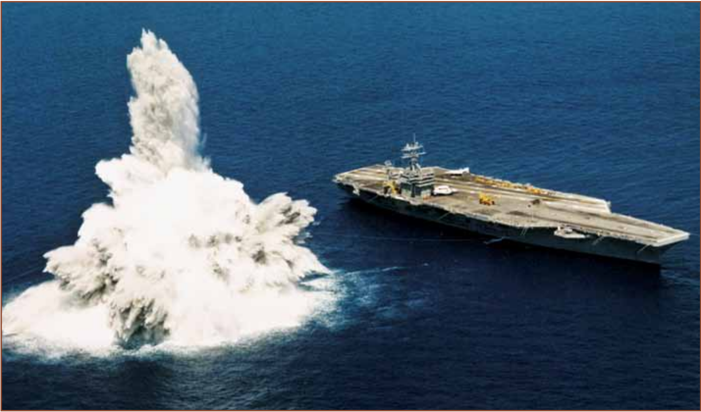
Above: The USS Theodore Roosevelt (CVN 71) undergoes open-ocean shock trials. Such events are costly to the Navy, and CREATE uses modeling and simulation software to predict the effects of underwater explosions, shock effects and damage resulting from such events.
