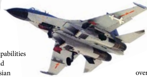
J-11B fighter armed with PL-8 air-to-air missile
