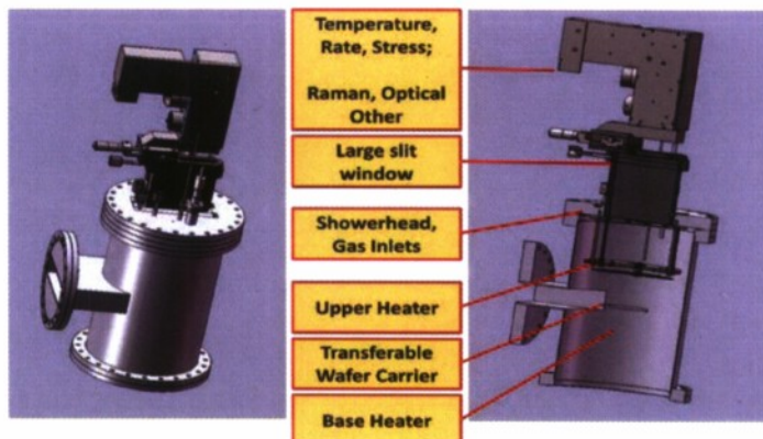
Figure 12 Schematic diagram of proposed production graphene reactor based upon existing Cornell reactor.
