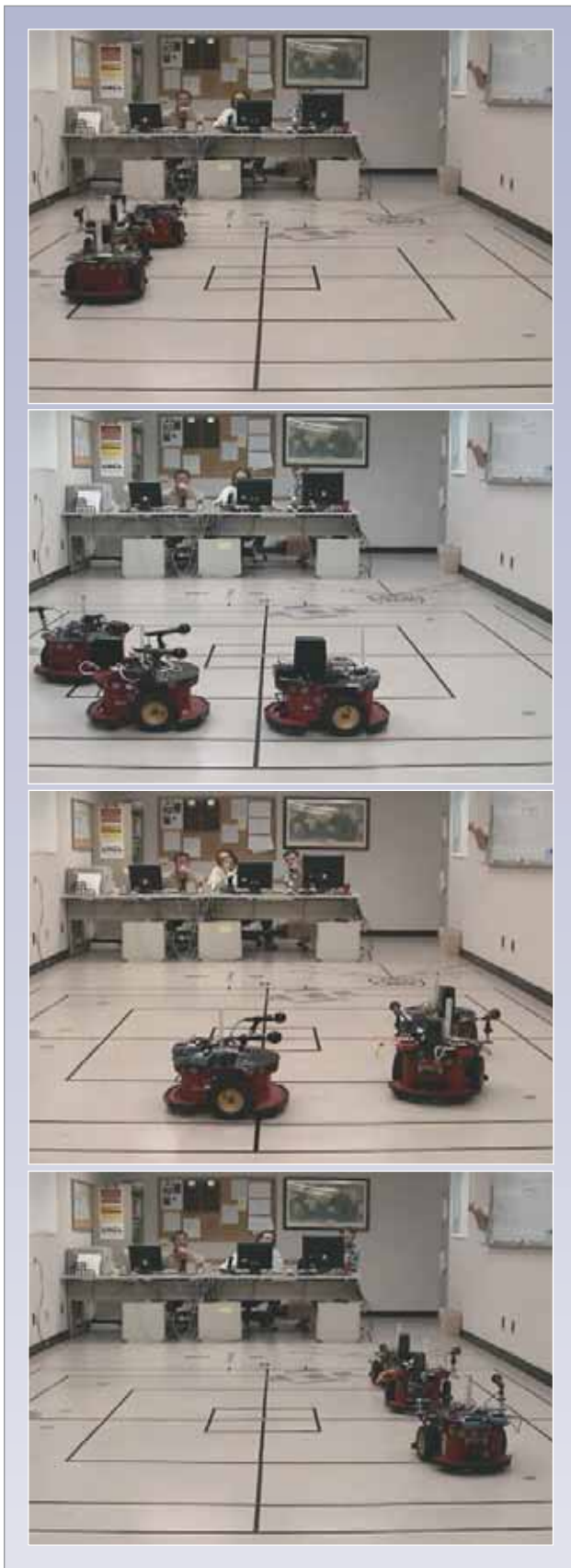
Figure 4. Formation maneuvering. Time lapse photos show three robots using their “ears” to follow each other in the lab.
