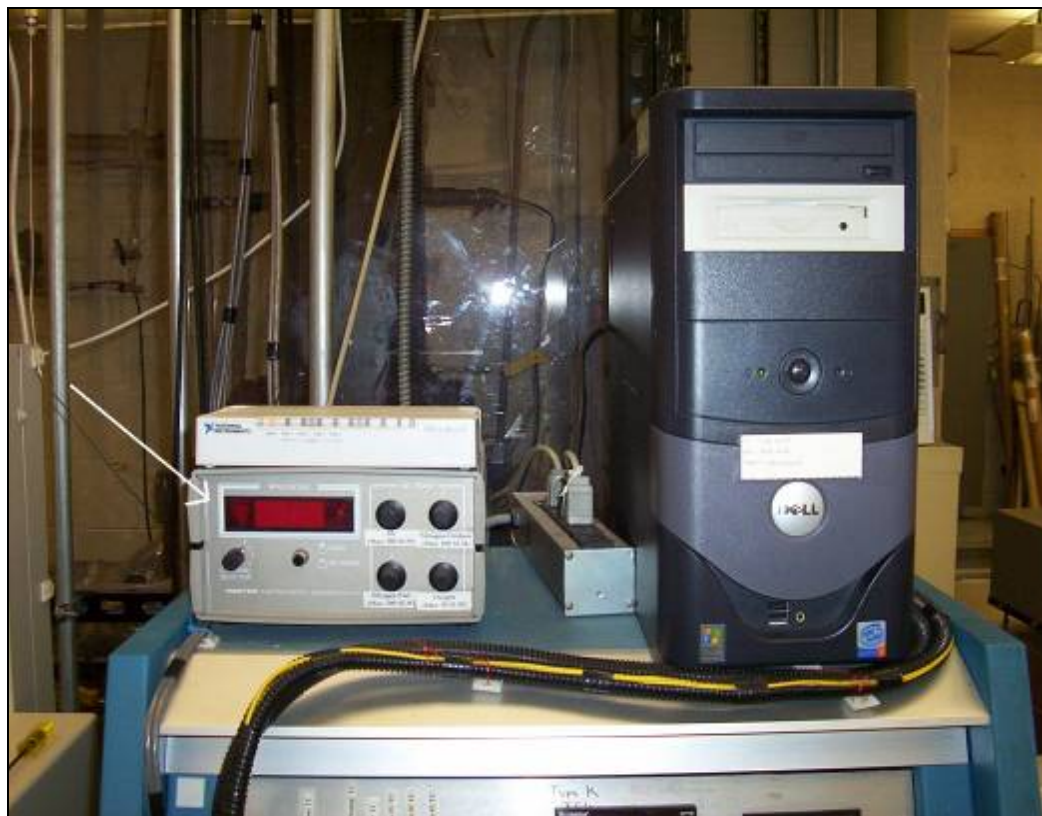
Figure A.2: Picture of PFR computer with the arrow identifying the PFR mass flow controller.
