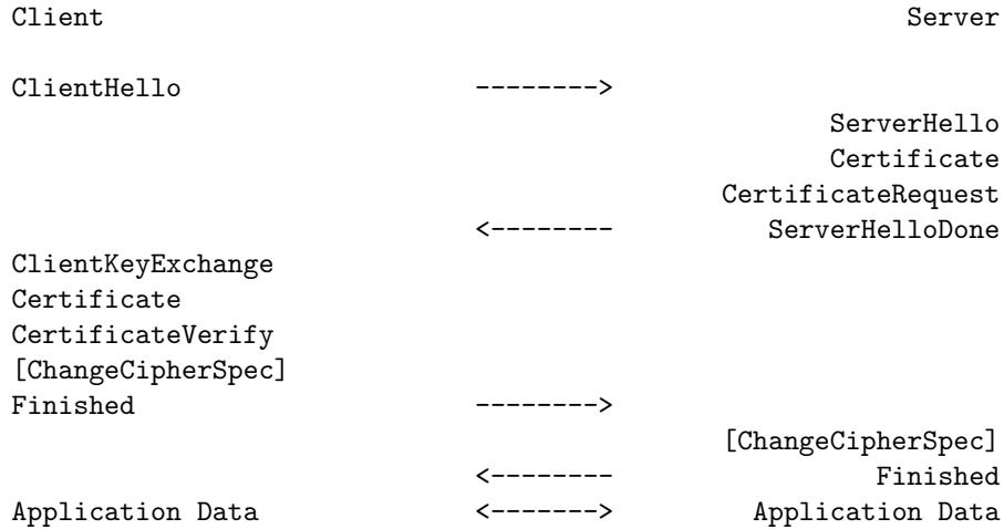
Figure 1-3: A Server-Client-Authenticating TLS Handshake.
