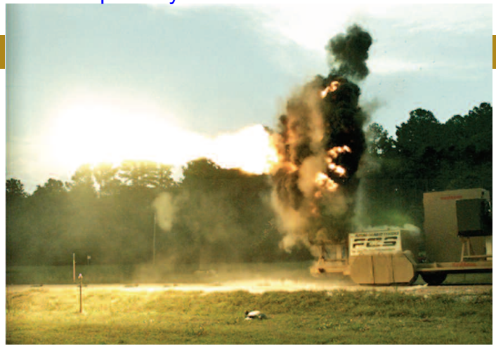
The rocket-propelled grenade defeat test here of the FCS Active Protection System for Manned Ground Vehicles was the first time that any vertical launch APS defeated an incoming rocket RPG while mounted on a moving vehicle. Photo by FCS
