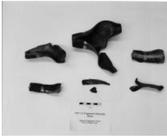
FIGURE 9. WARHEAD FRAGMENTS PRODUCED BY 105MM PROJECTILES LOADED WITH TNT
