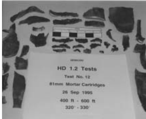
FIGURE 11. WARHEAD FRAGMENTS PRODUCED BY 81MM MORTAR WARHEADS
