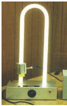
Figure 2. Demonstration of a Plasma Antenna in the On-State. The Antenna Electrically disappears when De-energized.[3] (Reprinted with permission from [3]. ©2008 American Institute of Physics.)
