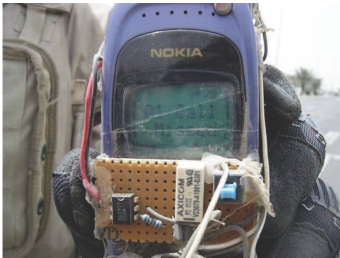
Figure 7. Cell phones can be used to detonate radio-controlled IEDs. (Note the one missed call.) JIEDDO's Counter Radio-Controlled Electronic Warfare vehicle-mounted, man-portable and fixed-site jamming systems prevent these devices from detonating. (Photo provided courtesy of JIEDDO)
