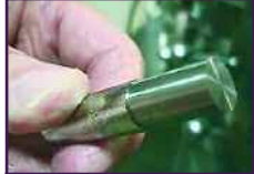
Left: A directionally solidified Galfenol alloy shown with a machined surface. Photo by James Restorff, NSWC Carderock Division.
