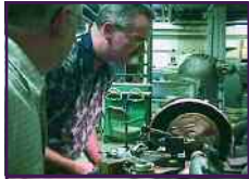
Left: Carderock Division's Scott Hoover machines a rod of a directionally solidified Galfenol alloy with Arthur Clark of Clark Associates looking on. Photo by James Restorff, NSWC Carderock Division.
