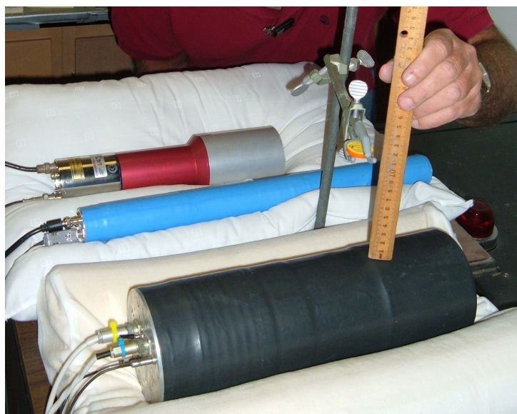
Figure 1 HPXe Test Detector (Front) during Test Series at UC-Irvine
