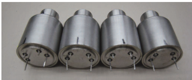
Figure 1. LCCM thermal battery prototypes.
