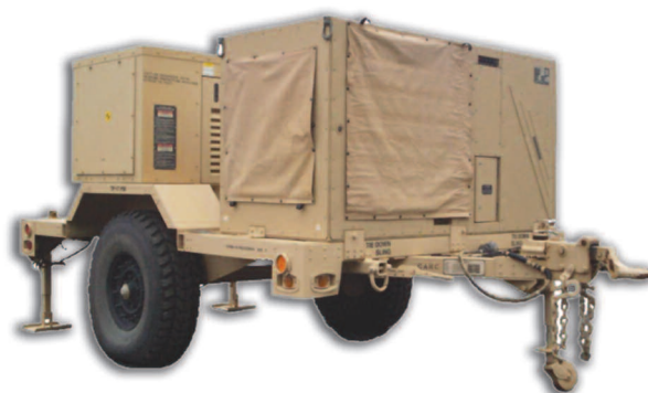
Figure 1. Integrated trailer-environmental control unit-generator.
