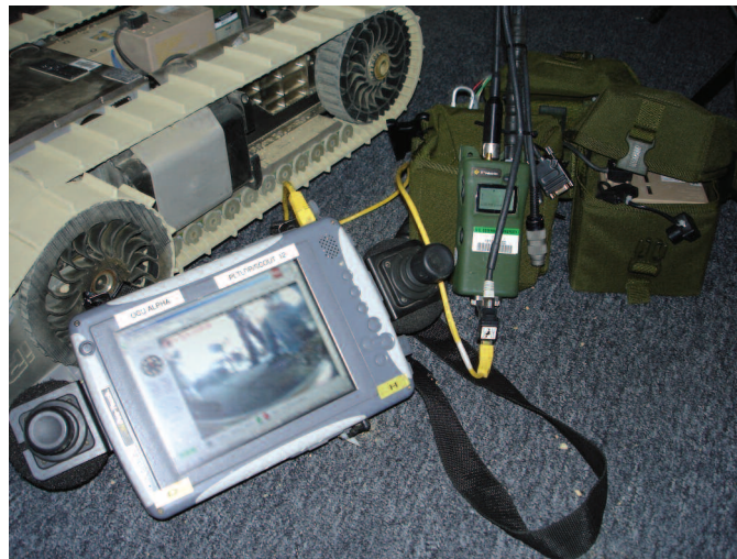
Figure 2. ARL OCU modified to use WSRT.
