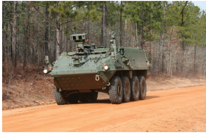
A Stryker is driven robotically through the Fort Gordon, GA, range during testing. Increased power demand on vehicles creates excessive heat, which can shorten component life and increase the burden on vehicle crews when cabin temperatures rise uncomfortably, placing further electrical demands on the system for cooling. (US Army photo by Larry Edmond)
