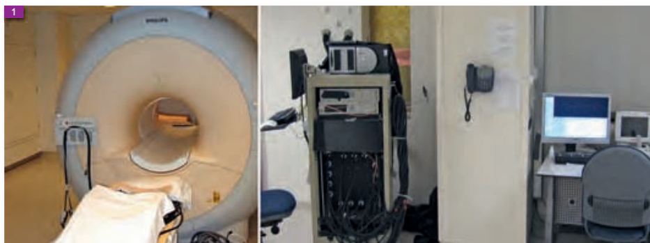
Figure 1. View of the MR guided NIRS breast interface attached to the breast coil on the MR table (left). Optical instrumentation and MR console (right).
