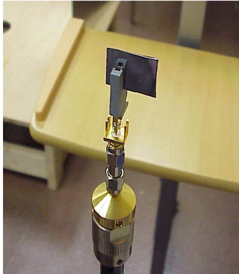
Fig. 8. Antenna support by two feeding electrodes.
