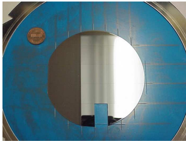
Fig. 7. A Si wafer cut into single die patches 20×13mm in size.
