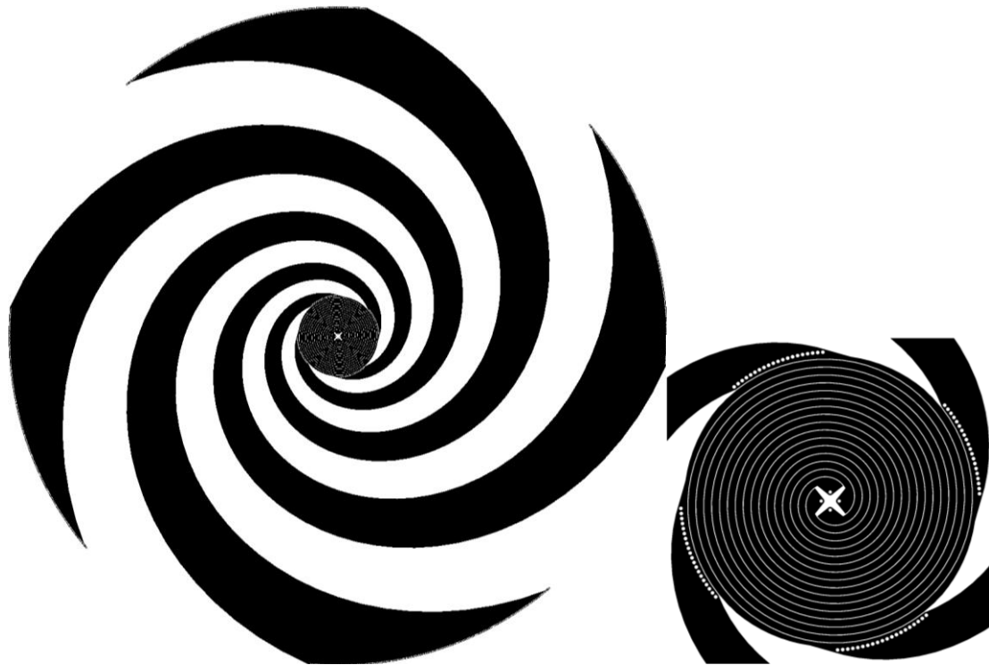
Fig. 16. Fabricated spiral antenna geometry. Full spiral geometry (left) and magnified transition region (left) images.
