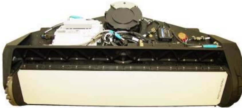
Figure 3.4.1-2. X-band Satellite-on-the-Move (SOTM) Antenna Subsystem
