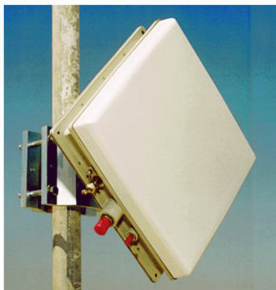
Figure 3.1-1. 38 GHz Point-to-Point CTS Antenna (with Exploded View)
