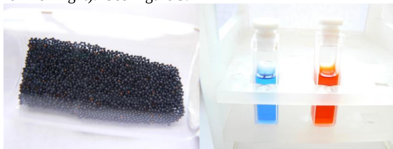
Figure 5. Fe(III) –Amberlyst resins and solutions of [\text{Fe}^{\text{III}}(\text{phen})_3]^{3+} (left) and [\text{Fe}^{\text{III}}(\text{phen})_3]^{2+}
