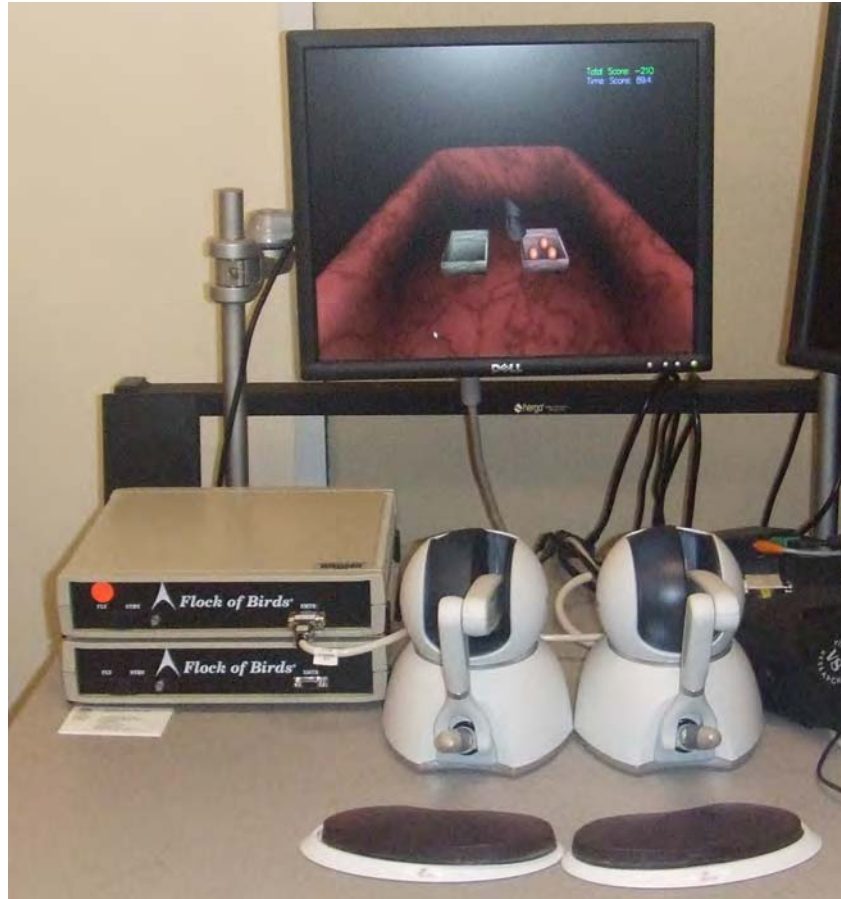
Figure 1. The VRMSS laparoscopic trainer for grasping, lifting & grasping and coordination skills is shown with dual force-feedback controllers.
