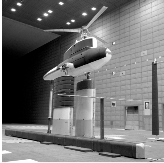
Fig. 1. Isolated XV-15 Rotor on the Rotor Test Apparatus in the 80- by 120-Foot Wind Tunnel.
