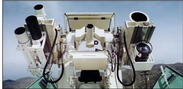
Figure 2. The KTM with the operator seat and multiple cameras.
