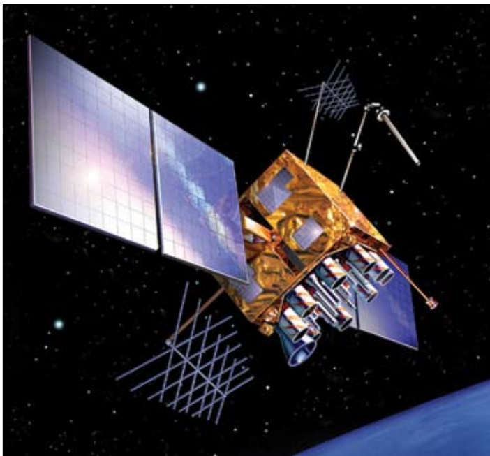
Figure 3. The Global Positioning System (GPS) IIRM satellites allow users equipped with a GPS receiver to determine velocity and worldwide position—latitude, longitude, and altitude—within a few meters. Both position data and velocity are given at a precise reference time. The GPS constellation works in concert with ground receivers to give precise location information to military and civilian users anywhere in the world. GPS provides such service as situational awareness and precision weapons guidance for the military. It is also an information resource supporting a wide range of civil, scientific and commercial functions—from air traffic control to the Internet—with precision location and timing information.
