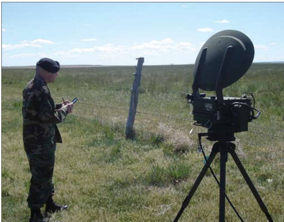
SrA Matthew Burke verifies directional data while setting up the man-portable surveillance target acquisition radar (MSTAR) for use within Malmstrom's missile field.
