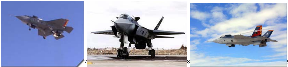
Figs 3-5: Notice on the top of the fuselage, while performing a vertical landing or at slow airspeeds, the lift fan inlet air duct doors are open.
