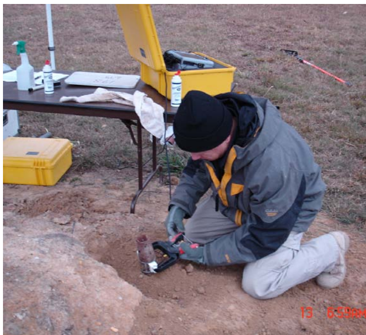
Figure 5. Explosives ordnance disposal (EOD) personnel clamping the acoustic sensors to a corroded 2.75-inch warhead.
