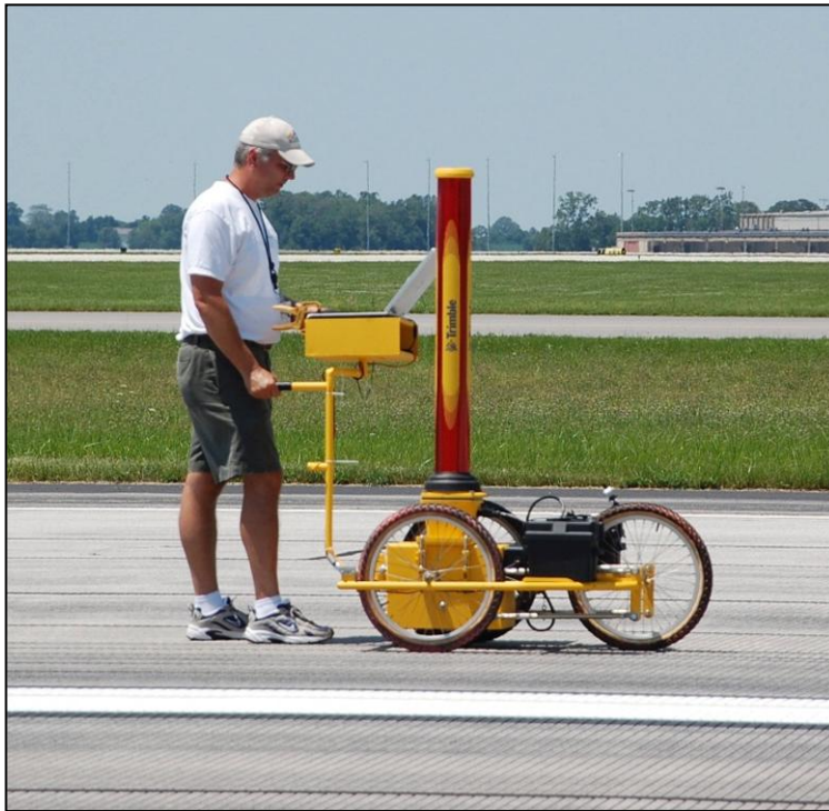
Figure 1: APR's Auto Rod and Level™ Profiling Device
