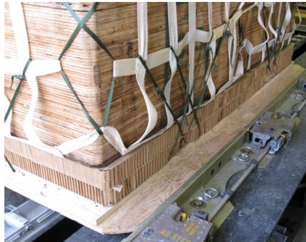
Figure 6. One-Time Use Plywood Platform Set Up in Roller Test Facility
