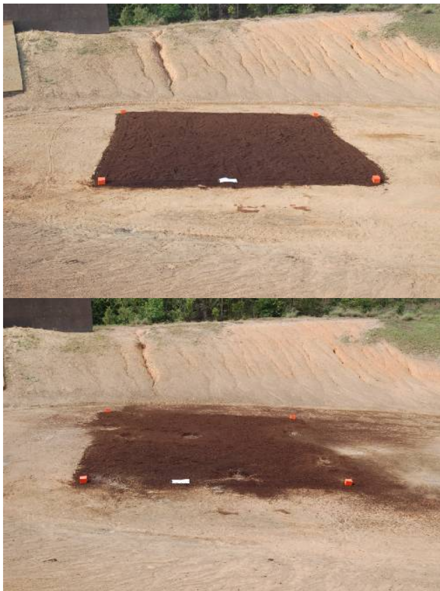
Figure 14. Photographs of PMSO treatment layer in Bay 1.
