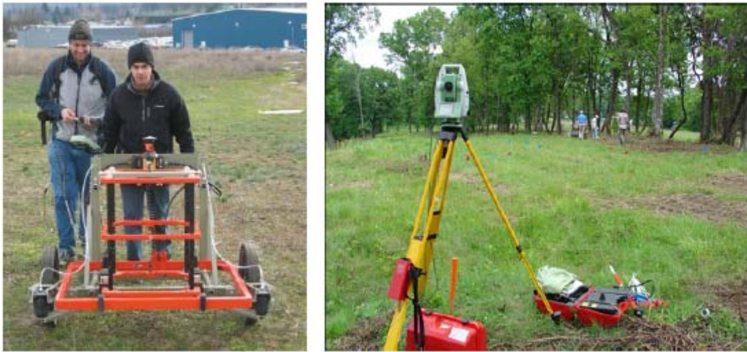
Figure 12. Equipment used at FLBGR including the modified EM63 cart (left) and the Leica RTS TPS1206 laser positioning system (right).
