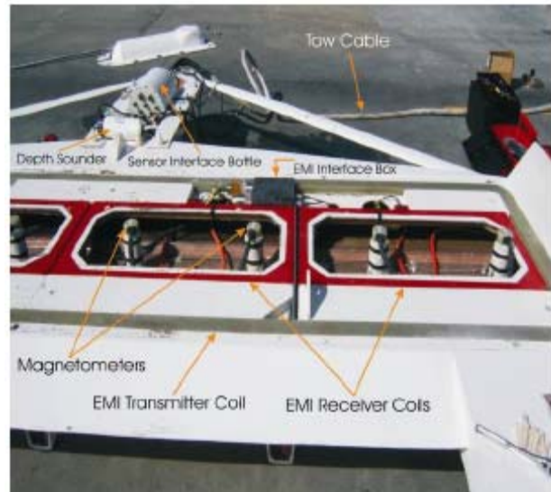
Figure 5. The marine sensor platform with hatch covers removed. Many of the system components are identified.
