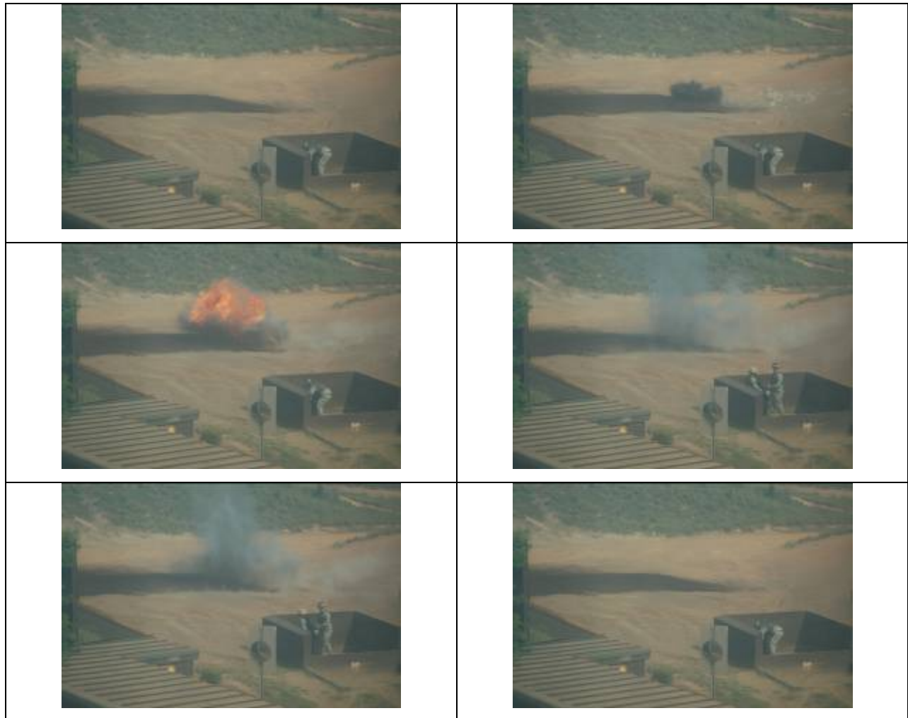
Figure 5.5-3. Photographs showing a grenade detonations on the PMSO layer in Bay 1.
