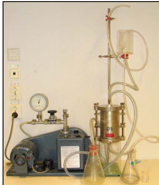
Fig. 6. Permeameter with vacuum device.
